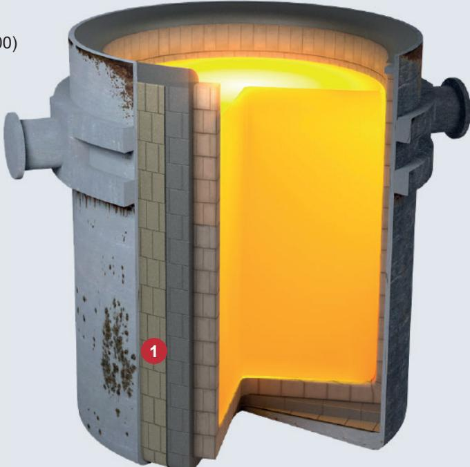
To meet the need for high mechanical strength, good thermal shock resistance and high service temperatures in steel ladles, Skamol has designed the SkamoSteel Vip 12 HS and SkamoSteel Vip 900 vermiculite-based insulation boards. These products help save energy and reduce costs.
